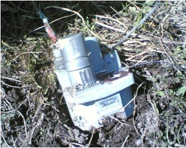
Fig. 15. Electromagnetic brake TЭM-4 for flap control found several meters behind the famous birch tree. Source: http://www.waronline.org
