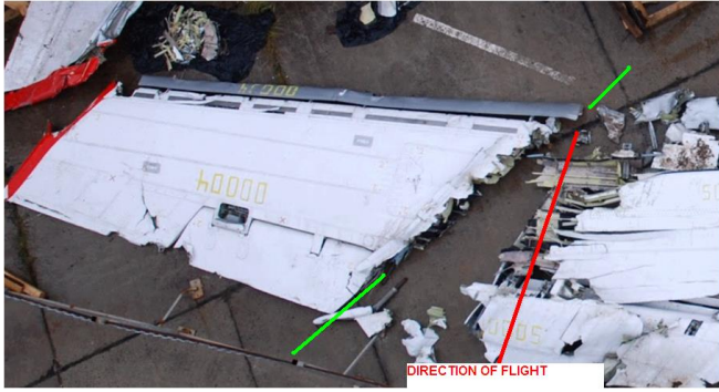
Fig. 21. The wing tip from P101 is cut along the line going from the natural division between the slats (point C) to the edge of the aileron. The crash engineer would warn that no good explanation can be given to the public for this issue .
