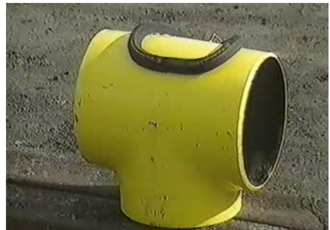
Fig. 15. The explosive can be formed in almost any shape. Here prepared to cut through a steel pipe [15].
