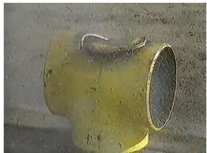
Fig. 16. The circular hole is cut with a sharp edge without throwing the parts around. Traces of the metal core of the directional explosive will deposit on the edges of the cut surfaces, in this case copper. Directional explosives can be found, where the metal core is aluminum matching the material of the wing better. The remainings of the plane will therefore contain valuable investigative information.
