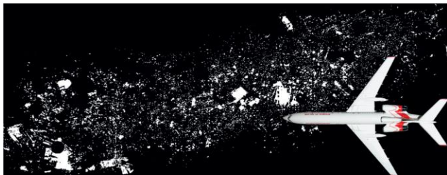
Fig. 2. A map of the debris found at the main crash site prepared for the Polish Archeologist report. The airplane in the bottom right corner shows the plane in the same scale [5].
