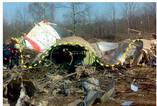
Fig. 5. Part of the inverted hull. It is clearly opened (yellow line and arrow) [5].
