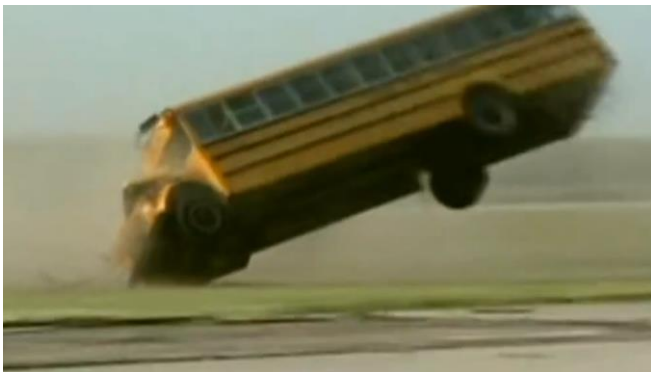
Fig. 9. This bus was pulled 40m behind one 747 engine blowing with the thrust power of the TU-154M. The 11 ton bus was immediately airborne and thrown another 30m - 40m downstream flipping around. See the YouTube video: https://www.youtube.com/watch?v=mj_bB6cUWCs
