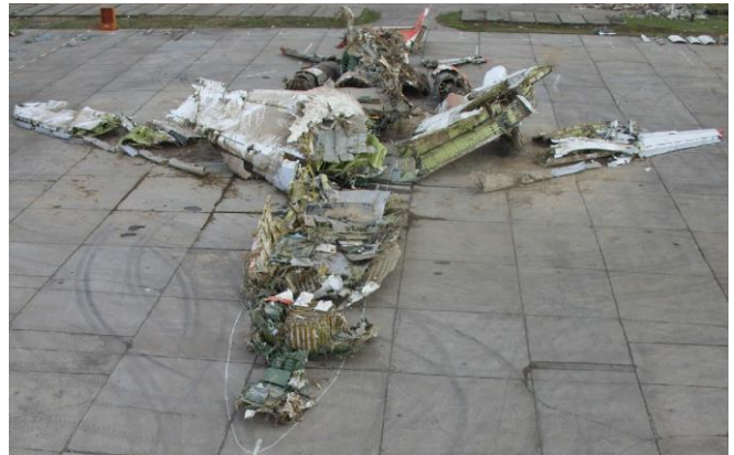
Fig. 24. The left and right wings show great similarity. Both are divided into: wing tip, center section in small pieces and the wing root. According to the official explanation the right wing was in free air all the time, and the left wing supposedly hit first a birch tree and later ploughed into the ground. The expected wing destruction should therefore be very different for the two sides left and right.
