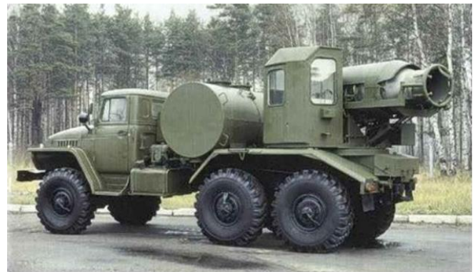
Fig. 25. An earlier serial produced version of the Russian truck based TMC65 fog generator.
