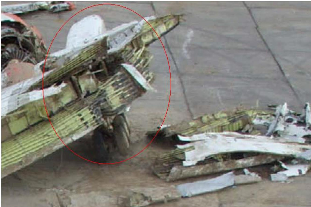
Fig. 28. The edge of the left wing root is bent backwards and shows clear sign of ground contact, so does the inner part of the slat, where the neighbour part of the slat shows no sign of ground contact. The bottom part of the middle section of the wing shows sign of ground contact, where the top part broken in fine sharp edged debris characteristic by explosion like described in Fig. 27. These observations agree with the hypothesis of wing loss by two explosions put forward in [2] and [7].
