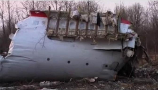
Fig. 6. The front bottom section below the president's salon. The entire top section is pulverized and the window section was thrown outwards most likely caused by the high internal pressure at the near ground explosion. Note the windows have not been in ground contact [7].
